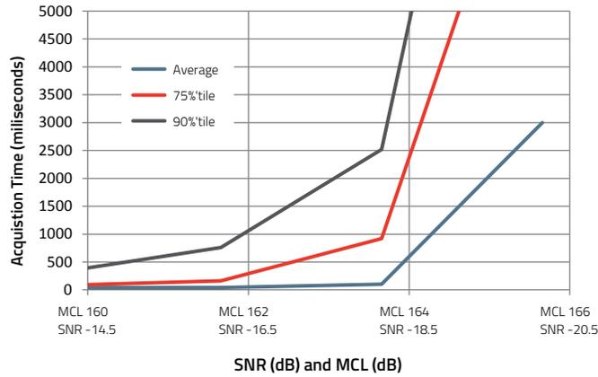
Figure 3: PBCH Acquisition Time versus SNR/MCL for "Keep Trying" Decoder
