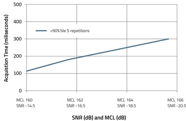
Figure 2: PBCH Acquisition Time versus SNR/MCL for Correlation Decoder
