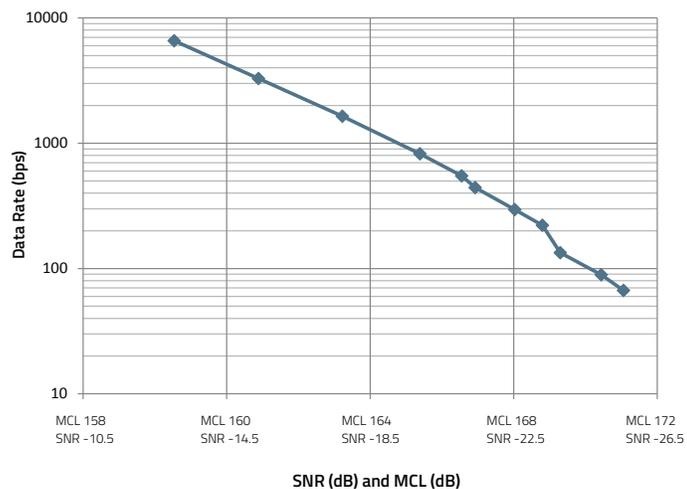
Figure 5: PDSCH data rate at 10% BLER versus the SNR/MCL
