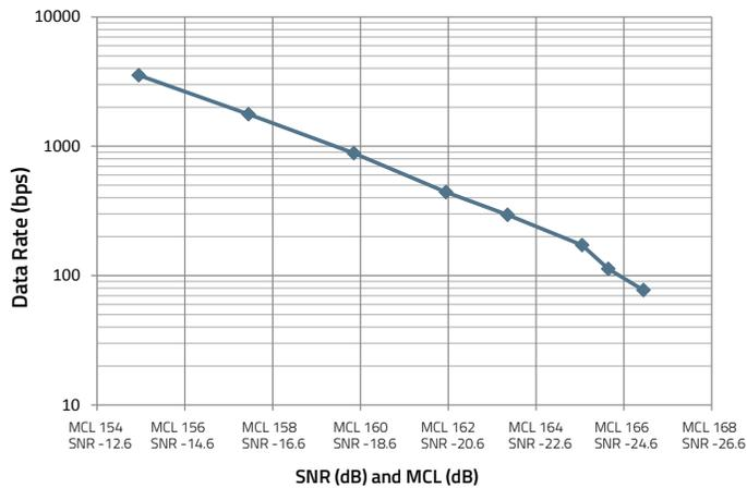
Figure 7: PUSCH data rate at 10% BLER versus the SNR/MCL
