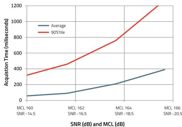
Figure 1: PSS/SSS Acquisition Time versus SNR/MCL
